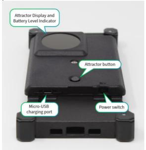
To set up this accessory, place the attractor on the back of the GoCheck Kids vision screening device.
