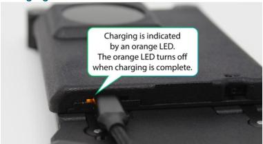
Use the micro-USB charge port with the provided micro-USB cable and USB charger. The Attractor will charge whether the power switch is On or Off. Charging is indicated by an orange LED light next to the micro-USB port. The orange light turns off when charging is complete. The average time to full charge is 5-6 hours.
