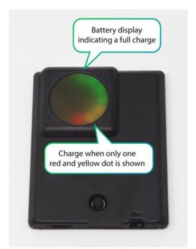
The battery level is briefly displayed when the power switch is turned on.
