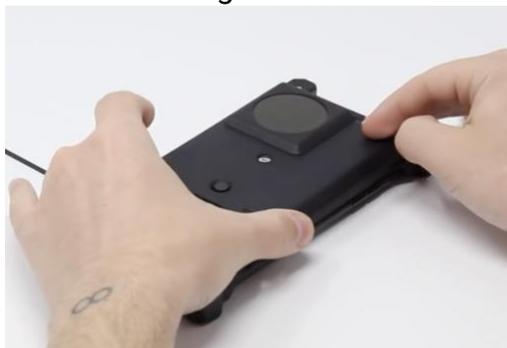
Using the supplied Allen key, tighten the screw until the attractor is properly secured. **Be sure not to overtighten the screw.**
