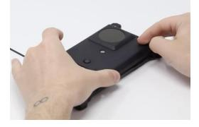
Using the supplied Allen key, tighten the screw until the attractor is properly secured. **Be sure not to overtighten the screw.**
