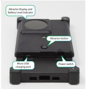
To set up this accessory, place the attractor on the back of the GoCheck Kids vision screening device.
